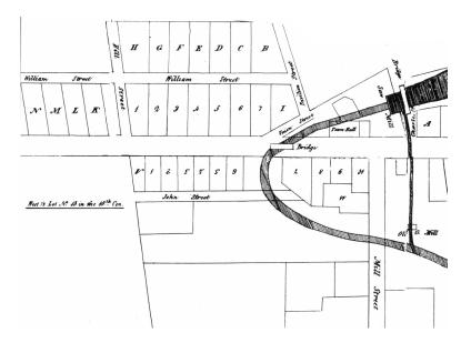
The water in the flume develops an amazing thirty horsepower as it drops seven metres from the dam at Charles Street to the small reaction turbine (a waterwheel mounted horizontally, rather than vertically) a hundred yards to the north-east. Few such mills in Ontario were sited as cleverly to take advantage of local topography.
