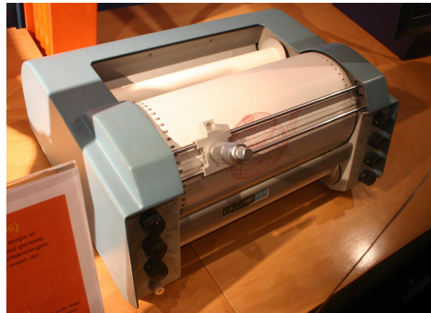
Figure 4: Two drawing machines. Top: Conté’s manual etching machine, 1800 [Courtesy CNAM]; bottom: the Calcomp 565, the first electronic drawing machine, 1958 [Courtesy Wikipedia]. (These and following images are grayscaled for print in TUGboat .)
