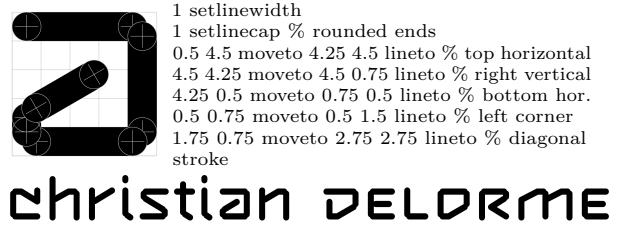
Figure 10: Left: an ‘a’ from Delorme; right: corresponding PostScript instructions [47]; below: Delorme’s name in his font.
