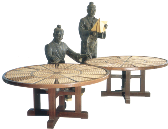
Figure 2: A model of Wang Zhen's revolving table for typesetting
