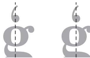
Figure 4: The optical axis of a glyph does not necessarily coincide with the geometric center of the glyph. Compare the corrected placement of the accent in gcommaaccent (left) with the default one (right).
